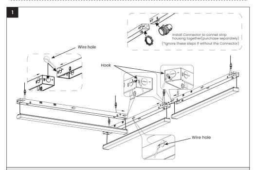
Use a screwdriver to pry open the Hook and open the Wire hole. Insert the hook into the hole in the direction of the arrow.
